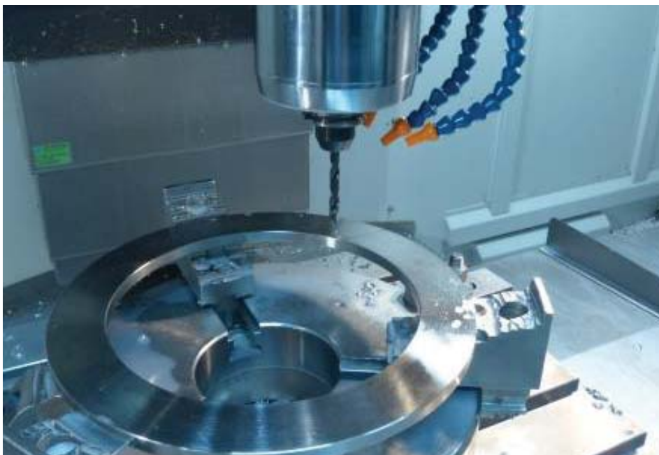
The WDO SUS carbide drill from OSG in use: Besides 1.4462 other stainless steels are processed and, according to Peter Heinz, these are no match in terms of problematic machining for the master class.
