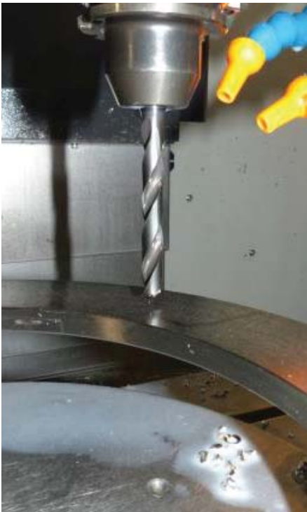
Lower cutting forces and less friction to reduce cutting temperature, a new chamfer design to allow lower feed rates and optimal chip forming are promised by OSG with the WDO SUS.
